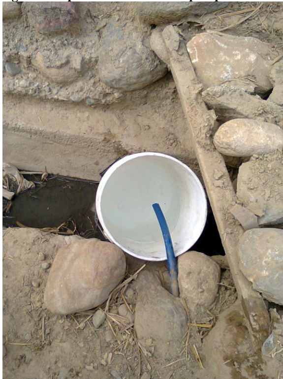
Figure 10: Water collection from existing tube well with discharge less than 1 liter per minute
